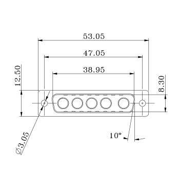
DESCRIPTION: 5W5 // M // CONNECTOR BODY FOR CRIMP CONTACTS
