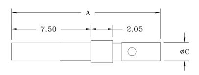
7.0MM RECOMMENDED WIRE STRIP DISTANCE. REFER TO ASSEMBLY SPECIFICATION FOR EXACT REQUIREMENTS (IPC/WHMA-A-620 AS AN EXAMPLE).
