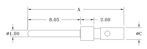
7.0MM RECOMMENDED WIRE STRIP DISTANCE. REFER TO ASSEMBLY SPECIFICATION FOR EXACT REQUIREMENTS (IPC/WHMA-A-620 AS AN EXAMPLE).
