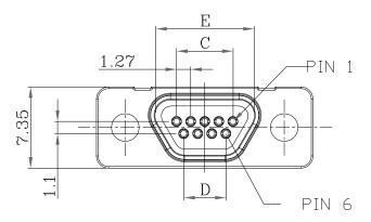
USE ABOVE FRONT FACE DIMENSIONS FOR PCB LAYOUT DESIGN. Ø0.8mm HOLE SIZE IS RECOMMENDED.
