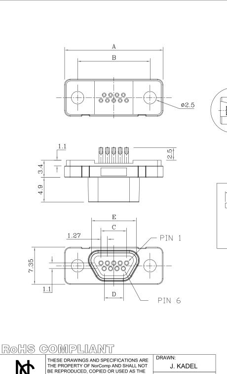
DESCRIPTION: SOLID BARREL MICRO-D // SOLDER CUP // FEMALE
