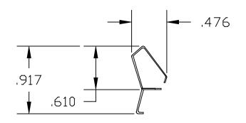
Spring Clip = 160-000-008R0S1 (2 required per connector assembly)
