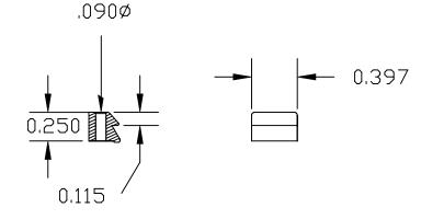
Latch Lock = 160-000-007R0P1 (PLASTIC) Latch Lock = 160-000-007R0M1 (METAL) Supplied 1 per (2 required per connector assembly)
