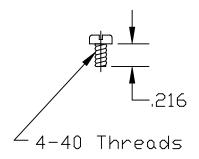
Mounting Screw = 160-000-009R0S1 (2 required per connector assembly)
