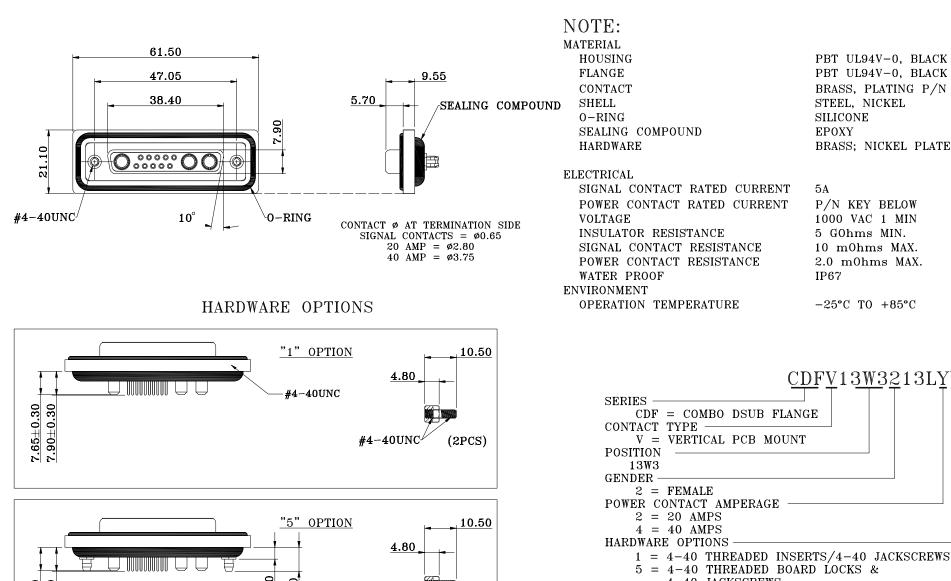
2.0 m0hms MAX. IP67 -25°C TO +85°C CDFV13W3213LYYY CDF = COMBO DSUB FLANGEV = VERTICAL PCB MOUNT
