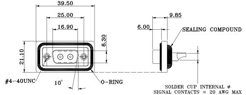
SULDER CUP INTERNAL  $\emptyset$ SIGNAL CONTACTS = 20 AWG MAX 20 AMP =  $\emptyset$ 2.70 (12AWG MAX) 40 AMP =  $\emptyset$ 4.60 (8AWG MAX)
