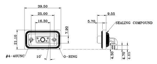
CONTACT Ø AT TERMINATION SIDE SIGNAL CONTACTS =  $\emptyset$ 0.65  $20 \text{ AMP} = \emptyset 2.80$  $40 \text{ AMP} = \emptyset 3.75$
