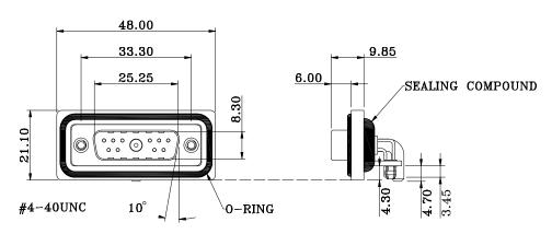
CONTACT Ø AT TERMINATION SIDE SIGNAL CONTACTS =  $\emptyset$ 0.65  $20 \text{ AMP} = \emptyset 2.80$  $40 \text{ AMP} = \emptyset 3.75$
