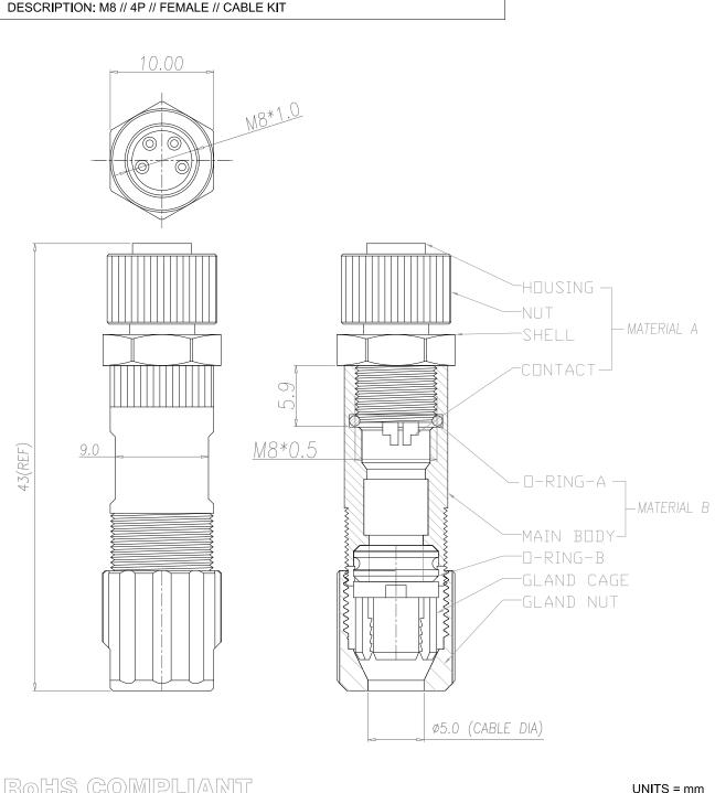
NOTE: MATERIAL A: HOUSING PBT UL94V-0, BLACK CONTACT BRASS, 10u"GOLD NUT ALUMINUM ALLOY, NICKEL ALUMINUM ALLOY, NICKEL SHELL MATERIAL B MAIN BODY ALUMINUM ALLOY, NICKEL O-RING A EPDM BLACK O-RING B NBR BLACK GLAND CAGE PA66 WHITE GLAND NUT PPS BROWN ELECTRICAL RATED CURRENT 3A VOLTAGE 60V INSULATOR RESISTANCE 100 MOhms MIN. CONTACT RESISTANCE 10 m0hms MAX.
