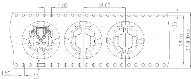
The tape size complies with the (EIA-481-D) specification requirements.
