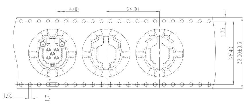
The tape size complies with the (EIA-481-D) specification requirements.
