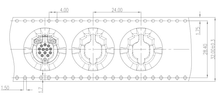
The tape size complies with the (EIA-481-D) specification requirements.
