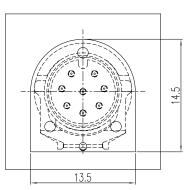
Component side (front view) Recommended keepout area on the circuit board
