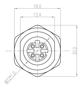
NOTE: MATERIAL HOUSING: PBT UL94V-0, BLACK CONTACT: **BRASS BRASS** NUT: SHELL: **BRASS** EPDM, BLACK D-RING 1: **FINISH** 10u" GOLD PLATED CONTACT: NUT: NICKEL PLATED SHELL: NICKEL PLATED **ELECTRICAL** RATED CURRENT: 4A RATED VOLTAGE: 250V 100 MOhms MIN. INSULATION RESISTANCE: CONTACT RESISTANCE: 10 mOhms MAX. WATER PROOF: IP67 **ENVIRONMENT OPERATION TEMPERATURE:** -40°C TD +85°C MAX WIRE AWG:
