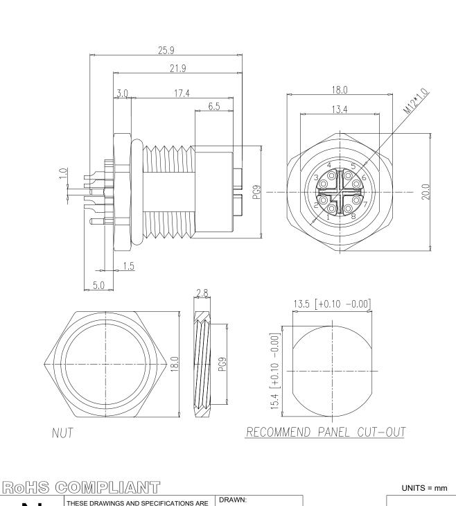
DESCRIPTION: M12 FEMALE - PANEL MOUNT (REAR) - 8 POS. - X-CODE - ROTATED
