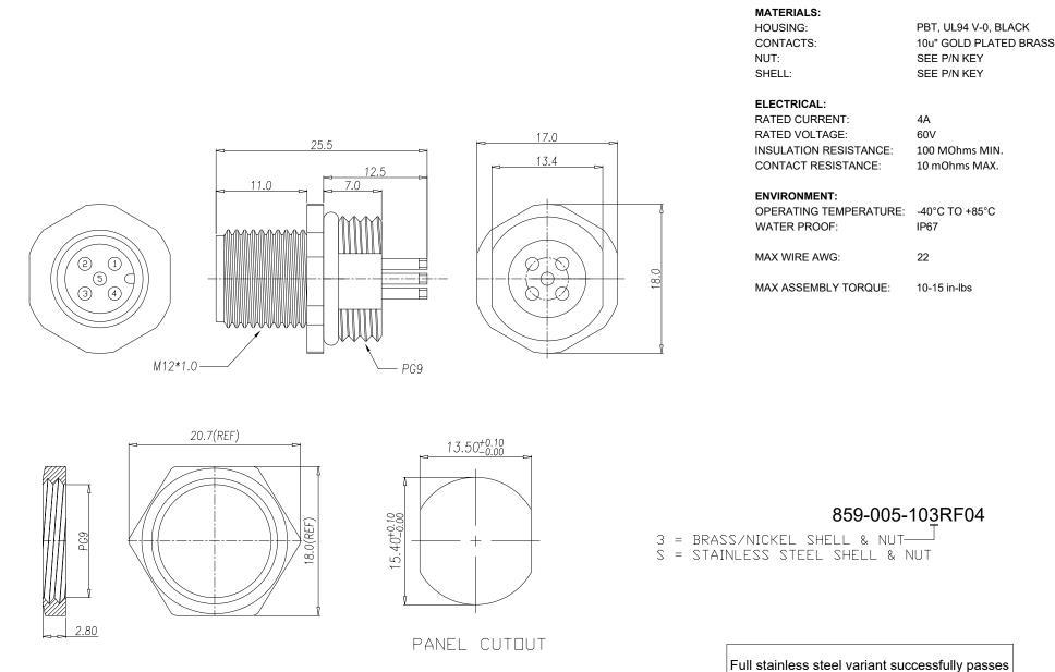
96-hour salt spray testing per ASTM B117
