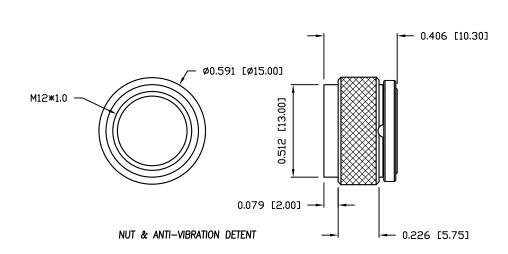
NOTE: MATERIAL HOUSING: PA66 UL94V-0, BLACK CONTACT: **BRASS BRASS** NUT: □-RING: EPDM, BLACK FINISH CONTACT: 10u" GOLD PLATED NUT: NICKEL **ELECTRICAL** RATED CURRENT: 4A 60V RATED VOLTAGE: INSULATOR RESISTANCE: 100 MOhms MIN. CONTACT RESISTANCE: 10 mohms MAX. WATER PROOF: IP67 **ENVIRONMENT OPERATION TEMPERATURE:** -40°C TD +85°C MAX WIRE AWG: 22 AWG
