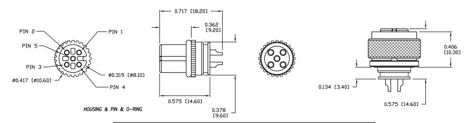
\*PLEASE NOTE THAT THE ANTI-VIBRATION DETENT IS MADE FROM PLASTIC AND IS NOT DESIGNED TO WITHSTAND MATING AND UN-MATING CYCLING; THIS WILL RESULT IN FAILURE OF THE ANTI-VIBRATION DETENT\*
