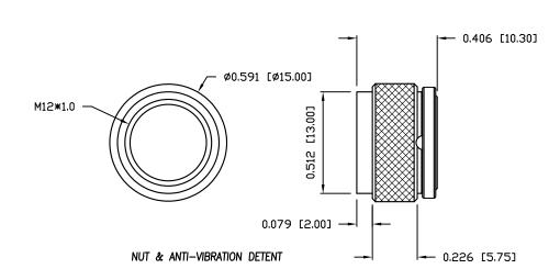
NOTE: MATERIAL HOUSING: PA66 UL94V-0, BLACK CONTACT: **BRASS BRASS** NUT: □-RING: EPDM, BLACK FINISH CONTACT: 10u" GOLD PLATED NUT: NICKEL **ELECTRICAL** RATED CURRENT: 4A 250V RATED VOLTAGE: INSULATOR RESISTANCE: 100 MOhms MIN. CONTACT RESISTANCE: 10 mohms MAX. WATER PROOF: IP67 **ENVIRONMENT OPERATION TEMPERATURE:** -40°C TD +85°C MAX WIRE AWG: 22 AWG
