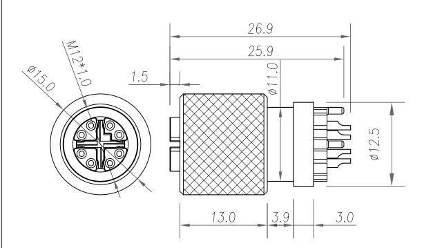
NOTE: MATERIAL HOUSING: PA66 UL94V-0, BLACK CONTACT: BRASS, 10u" GOLD SHELL: BRASS, NICKEL PLATED X-SHELL: ZINC ALLOY NUT: BRASS, NICKEL PLATED BACK SHELL: BRASS, NICKEL PLATED DRING: **EPDM ELECTRICAL** RATED CURRENT: 0.5A 50VAC/60VDC RATED VOLTAGE: INSULATION RESISTANCE: 100 MOhms MIN. CONTACT RESISTANCE: 10 mOhms MAX. WATER PROOF: IP67 ENVIRONMENT **OPERATION TEMPERATURE:** -40°C TD +85°C MAX WIRE AWG: 24
