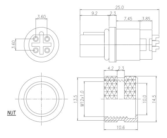
NOTE: MATERIAL HOUSING: PBT UL94V-0, BLACK CONTACT: BRASS SHELL: BRASS NUT: BRASS □-RING: EPDM, BLACK FINISH 10u" GOLD PLATED CONTACT: NICKEL UNDER PLATE: NUT: NICKEL SHELL: NICKEL ELECTRICAL RATED CURRENT: 4A RATED VOLTAGE: 250V INSULATOR RESISTANCE: 100 MOhms MIN. CONTACT RESISTANCE: 10 m□hms MAX. WATER PROOF: IP67
