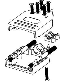
BACKSHELL MATERIAL: PLATING: JACKSCREWS: CLAMP SCREWS: CLAMPS: OPERATING TEMP: DIE-CAST ZINC ALLOY NICKEL STEEL:NICKEL PLATED STEEL:ZN PLATED ZINC DIE CAST -40°C TO+120°C
